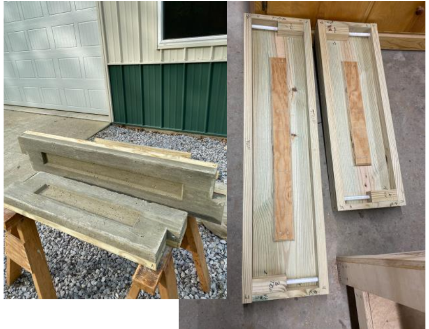
DWIGHT HOSTETTER Molds for concrete raised bed garden sides
