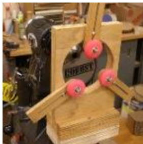
Steady Rest or Center Steady For turning larger pieces
