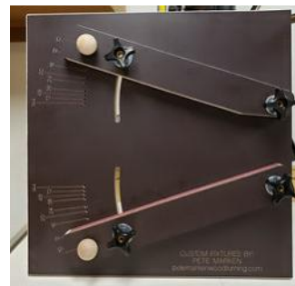
Wedge-less Sled for cutting segments
