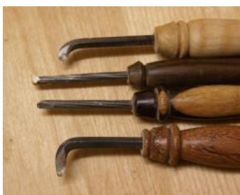
Mini Hollowing Tools Made with Allen Wrenches
