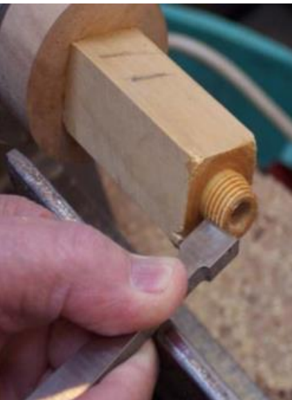
Threading the tenon on the top of the base section.
