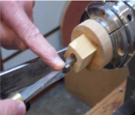
Threading the hole in the lid with the inside chasers.
