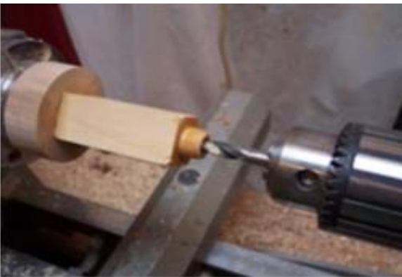
Drilling the 5/16" hole to hold the needles. It can be drilled before or after threading.
