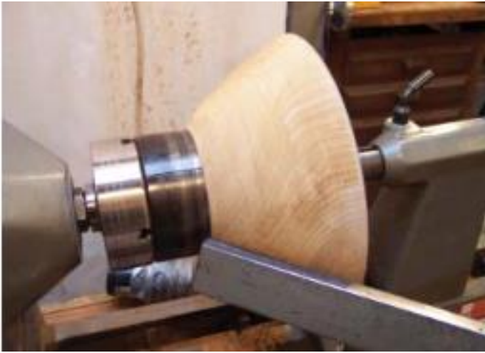
Turning the outside of the bowl when mounted in the Nova Chuck.
