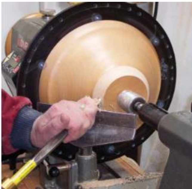
Turning the foot of the bowl. The tailstock was removed for final turning away of the little tenon in the center and for final sanding.
