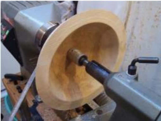
This cup-shaped live center doesn't mar the bowl's surface when used as support for the chuck.
