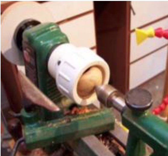
Picture 2. In this photo, the tail center is being used to align the ball on center before the chuck is tightened.
