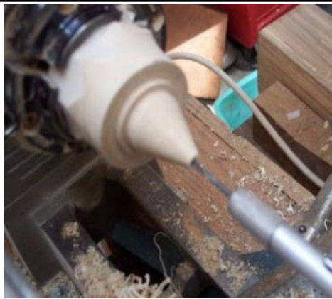
Photo 7. Drilling the 3/32" hole in the cone
