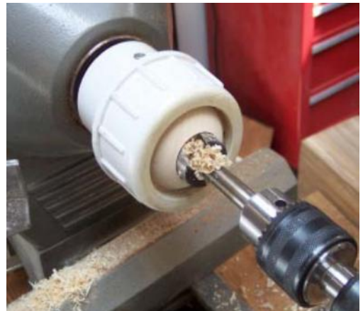
Photo 3. Drilling the 1-1/4" hole about 1/4" deep.
