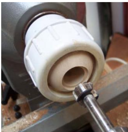
Photo 4. Drilling the 1" hole about 3/4 of the way through the ball.
