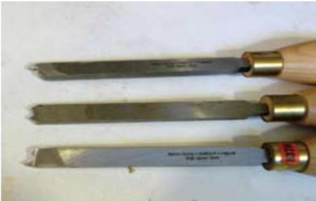
Figure 7. The Robert Sorby tools used in this project: (top to bottom) Right hand side tool, beading tool, and left hand side tool.
