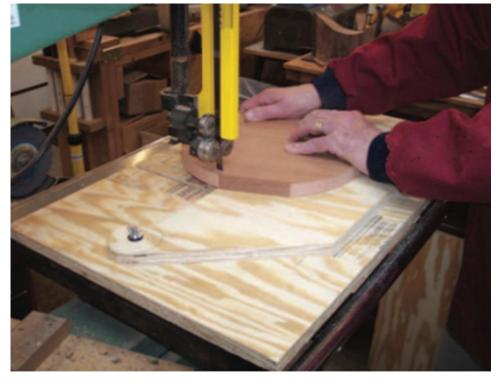
The Circle Cutting Jig being used to cut a round disk from a flat board. This rig worked best on flat boards because my bandsaw blade tended to wander a bit as the circle cutting process proceeded.
