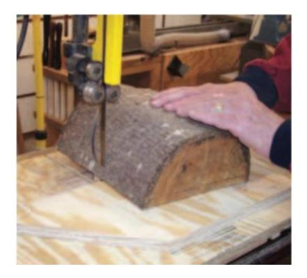
This certainly made it much easier to cut a 1/2 log section into a round circle than trying to use a cardboard disk to guide the cut.
