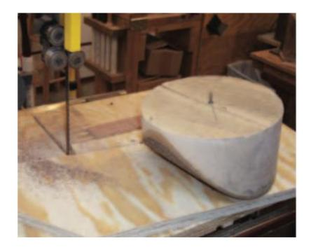
This photo shows the finished piece. Note the duplex nail sticking out of the bottom of the turning blank.
