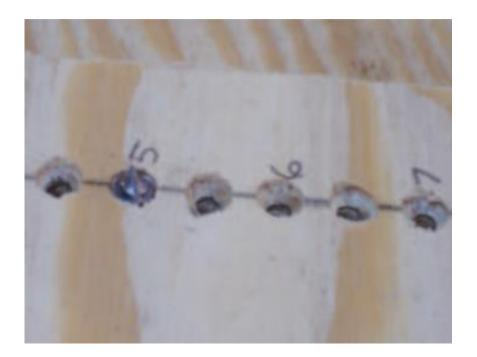
I made two different pivot pins: one shown in the five inch position in the above photo; the other was a bit longer for thicker blocks of wood. I used the short one to cut flat boards and the longer one to cut half log sections as shown below.
