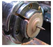
Once the epoxy has cured, the small size screw chuck is ready to use. Remount it into your chuck. Screw on your wood blank and turn to a shape of your choosing using gouge, skew and or scrapers. **Turning the wood to shape, in this case a neat knob.**
